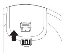
2. Flip the Retainer over so the tab is facing up, and slide the Retainer back into the Base Unit.
